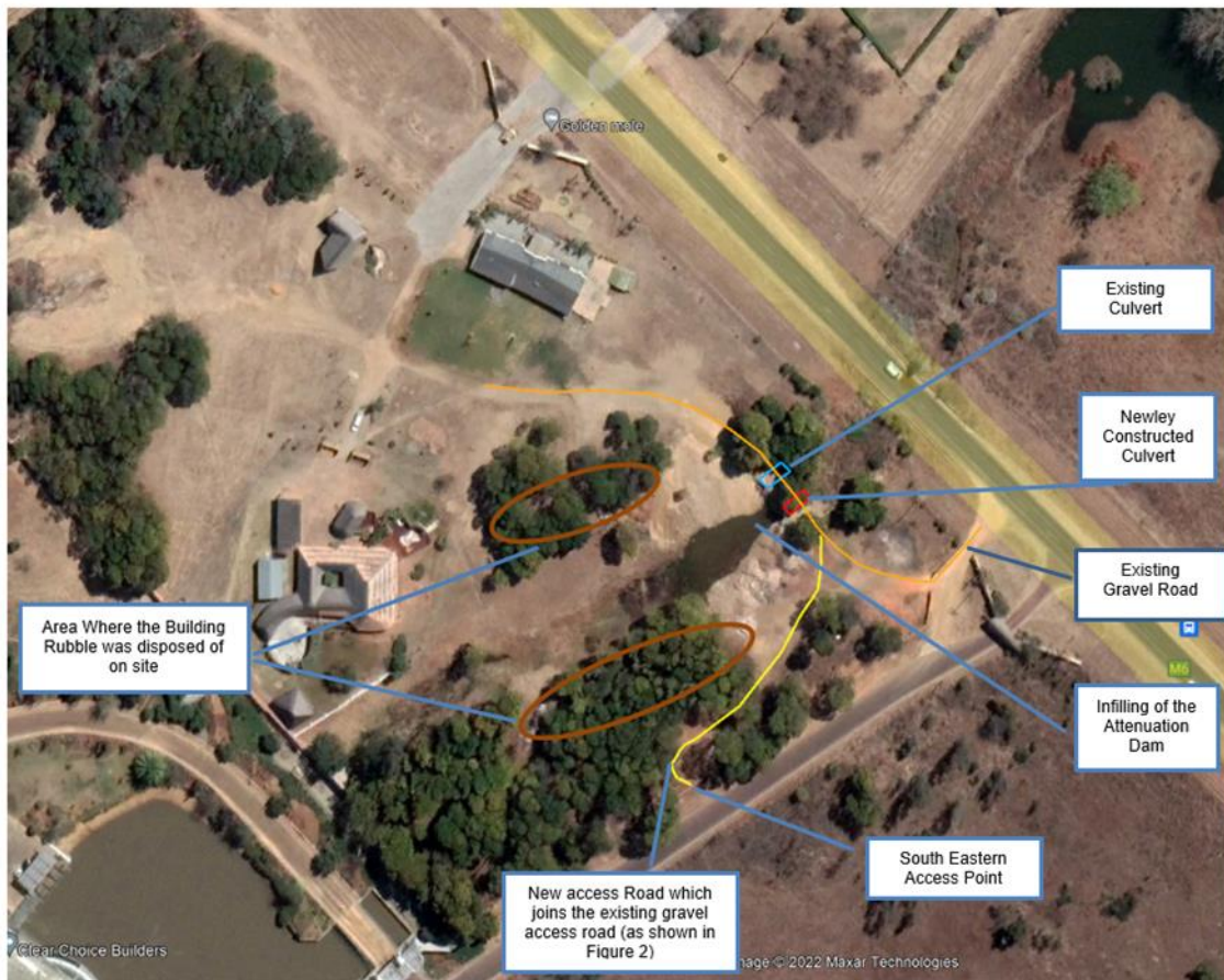
Figure 2:3 Google Earth Image (2021) showing the construction activities undertaken on site
