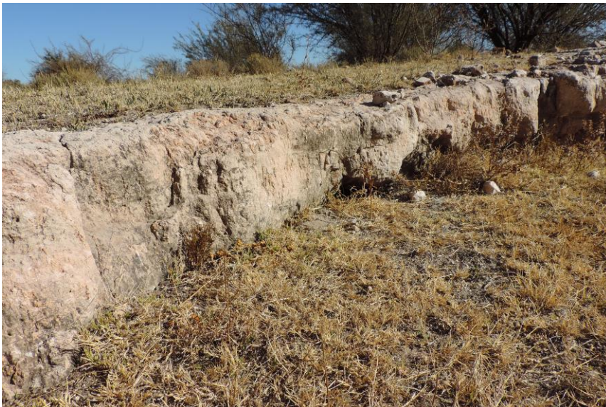
Figure 12 Photographic evidence of an exposed Coega soil profile on Portion 2 of the farm Murray 570
