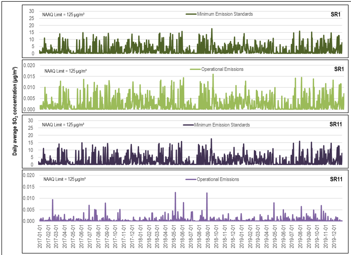
Figure 5-12: Time series of the daily SO 2 concentrations simulated at the nearest receptors
