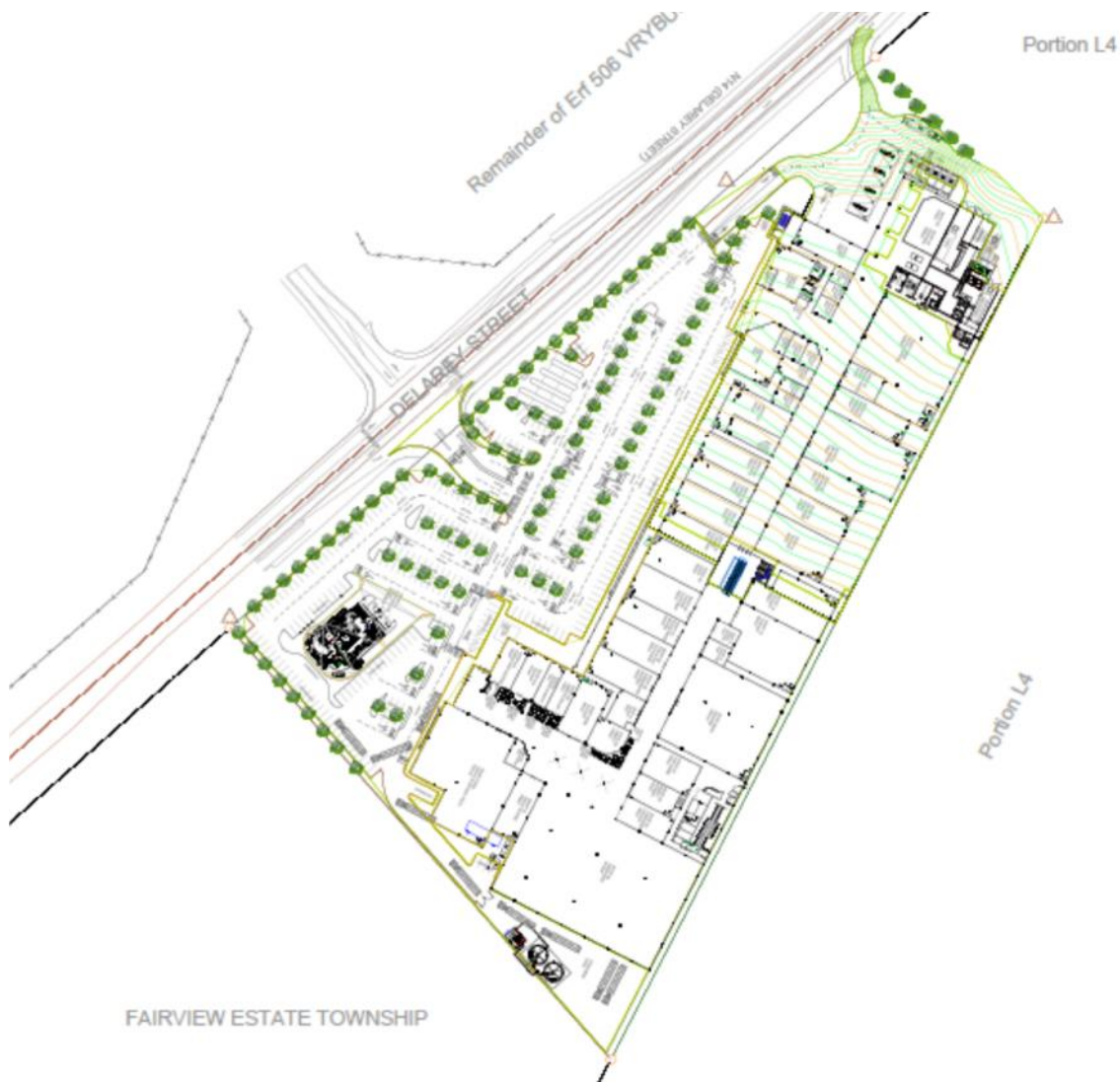
Bulk Earthworks – lower parking contours plot (BSM Consulting Engineers, 2022)
