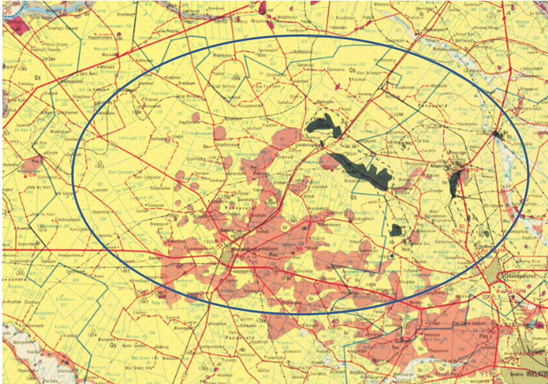
Figure 6-1: Geological map of the area around the Target area 1 indicated within the blue oval. Abbreviations of the rock types are explained in Table 2. Map enlarged from the Geological Survey 1: 250 000 map 2726 Kroonstad.
