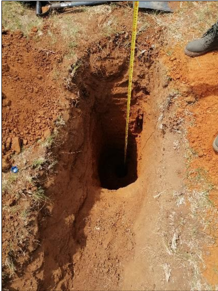
Photograph 1: Typical view of colluvium and ferricrete
