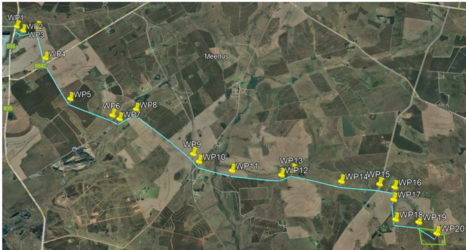
Figure 1-5: Water pipeline route - Preferred Alternative
