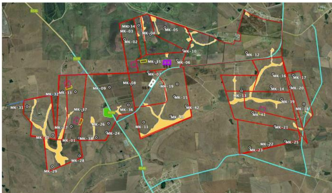
Figure 1-12: Current layout of the infrastructure in the Mukondeleli site in relation to habitat sensitivity on site (Ekotrust, 2022) (Key: Pink squares SS E = switching station E; White squares SS F = switching station F; Yellow rectangles = construction and batching sites; Pink squares = laydown areas; and Turquoise = Main roads)
