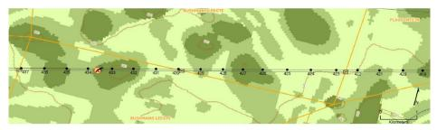
**Figure 1:** Example of an environmental sensitivity map in the context of a final overhead transmission and distribution profile.
