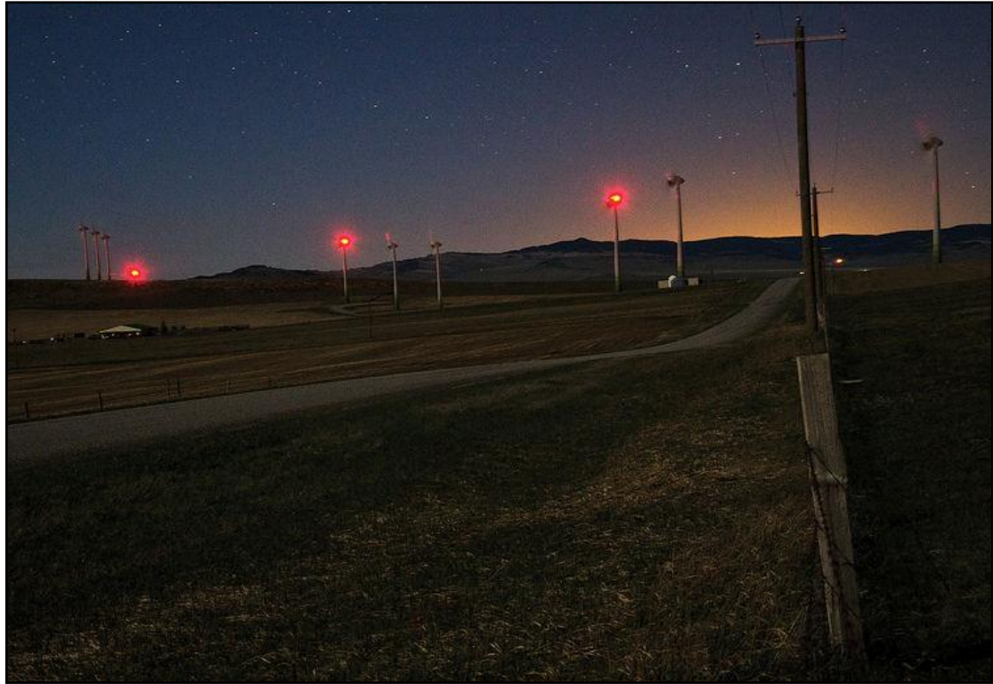
Figure 27: Aircraft warning lights fitted to the wind turbine hubs (Source: http://www.pinchercreekecho.com/2015/04/29/md-of-pincher-creek-takes-on-wind-turbine-lights. )
