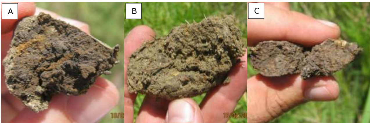
Figure 6. Examples of some of the wetland indicators found in the soil. Red mottles, haematite, ( A ) and yellow mottles, goethite, ( B ) form under fluctuating water table where the iron accumulates during redox. Soft plinthic showing a goethite nodule ( C ) - formed over many years of a fluctuating water table and an accumulation of iron and manganese mottles.
