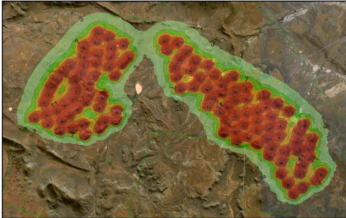
Figure 7-6: Change in ambient sound levels (Concawe model), contours of constant noise levels with a South-southeast wind blowing at 5 m/s (turbines marked as red dots, PSRs as green dots)
