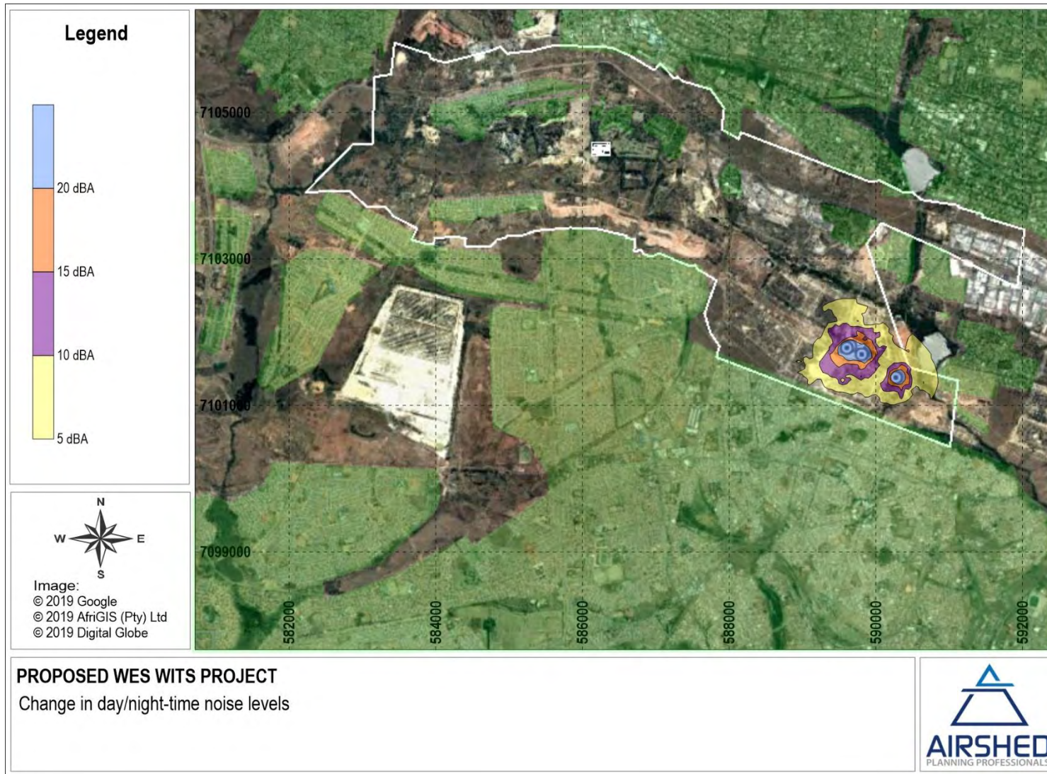
Figure 18: Simulated change in day/night time noise levels due to underground mining project activities
