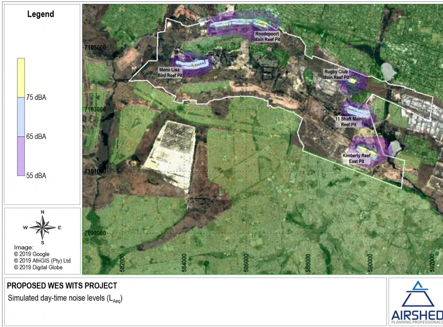
Figure 9: Simulated equivalent continuous day-time rating level ( L_{Req,d} ) for opencast mining project activities
