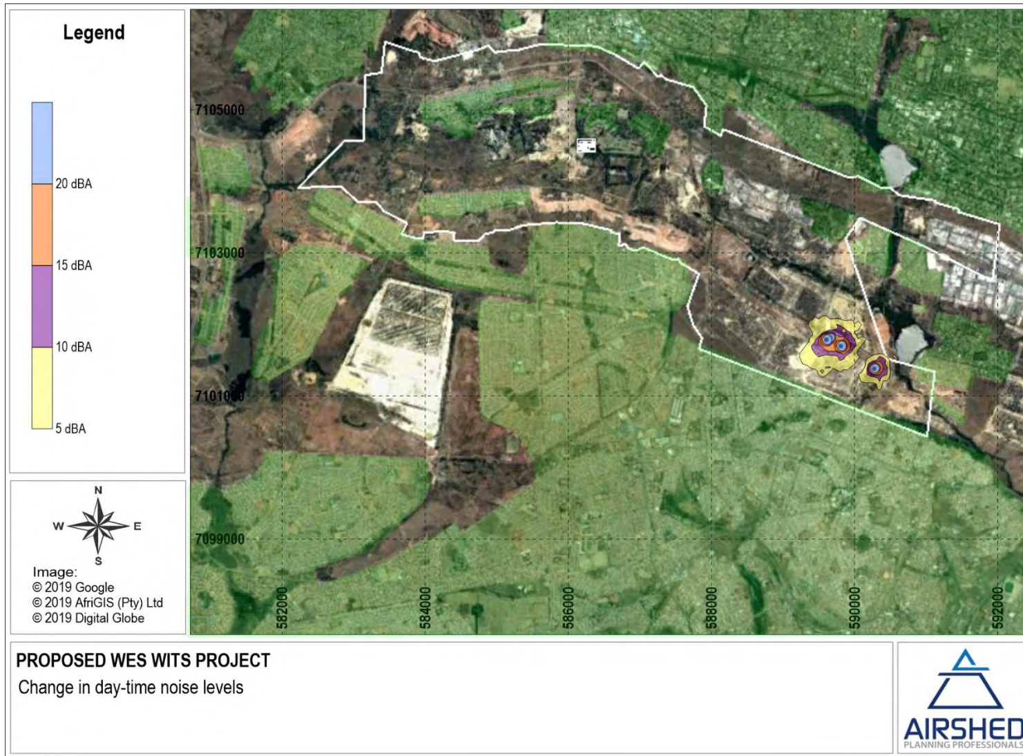
Figure 16: Simulated change in day-time noise levels due to underground mining project activities
