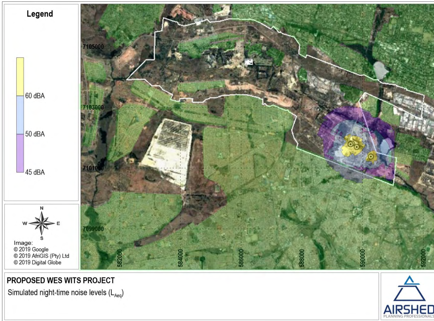
Figure 12: Simulated equivalent continuous night-time rating level ( L_{Req,n} ) for underground mining project activities
