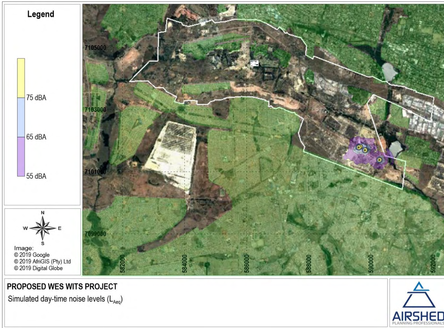
Figure 11: Simulated equivalent continuous day-time rating level ( L_{Req,d} ) for underground mining project activities
