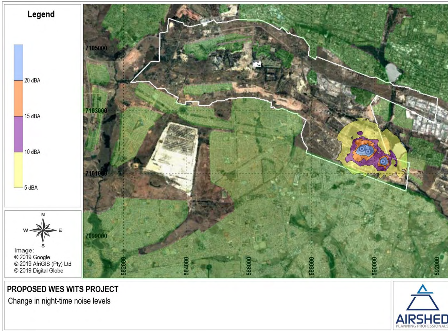
Figure 17: Simulated change in night-time noise levels due to underground mining project activities
