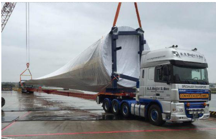
Figure 2.2: Example -Transport of Blades on extendible trailers
