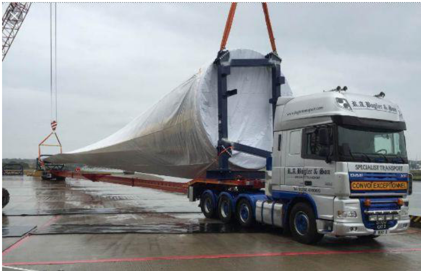
Figure 2-2: Example -Transport of Blades on extendible trailers
