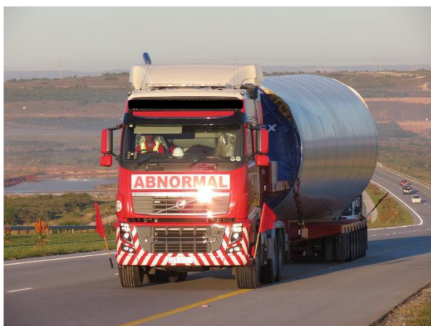
Figure 2-4: Example – Transportation of Tower Sections
