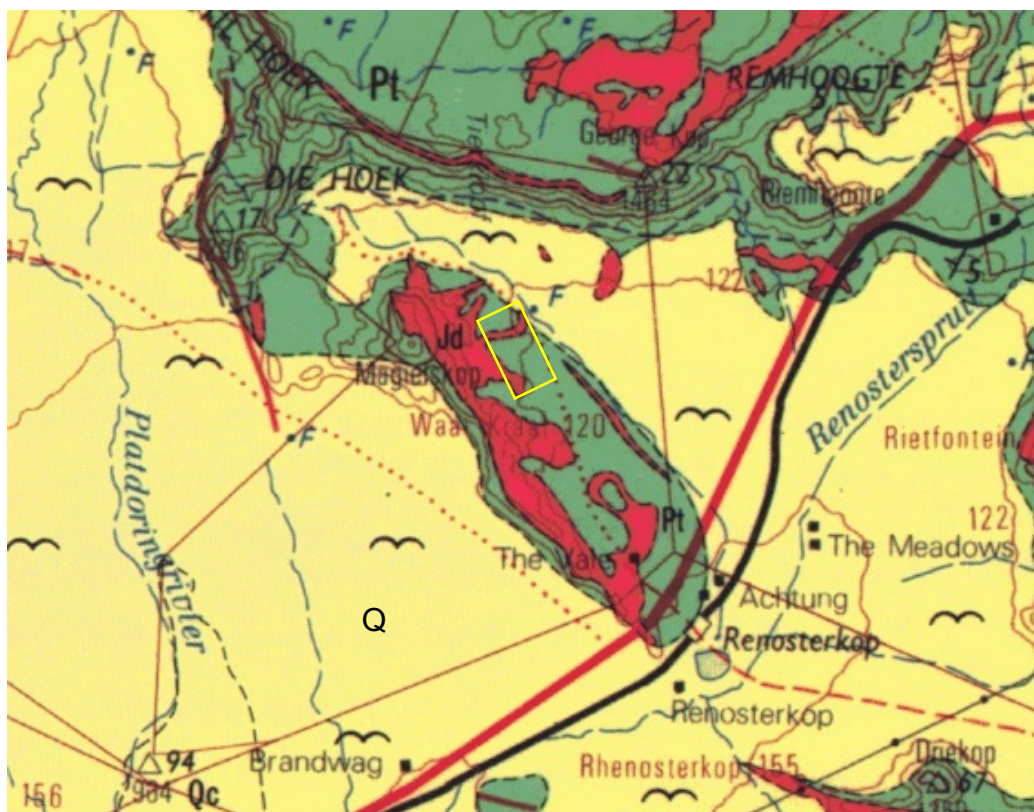
Figure 6: Geological map of the area around Farm Waai Kraal 120, with the location of the proposed project is indicated by the yellow rectangle. Abbreviations of the rock types are explained in Table 2. (Map enlarged from the Geological Survey 1: 250 000 map 3222 Beaufort West).
