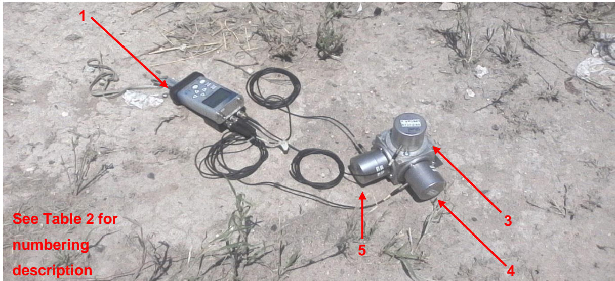
Figure 1: Illustration of test setup including seismic accelerometers and Svantec data logger
