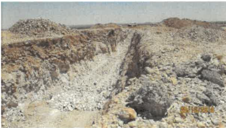
Photo 19: Typical Feldspar mining site. Note the steep side walls and the mining technique (trenching).
