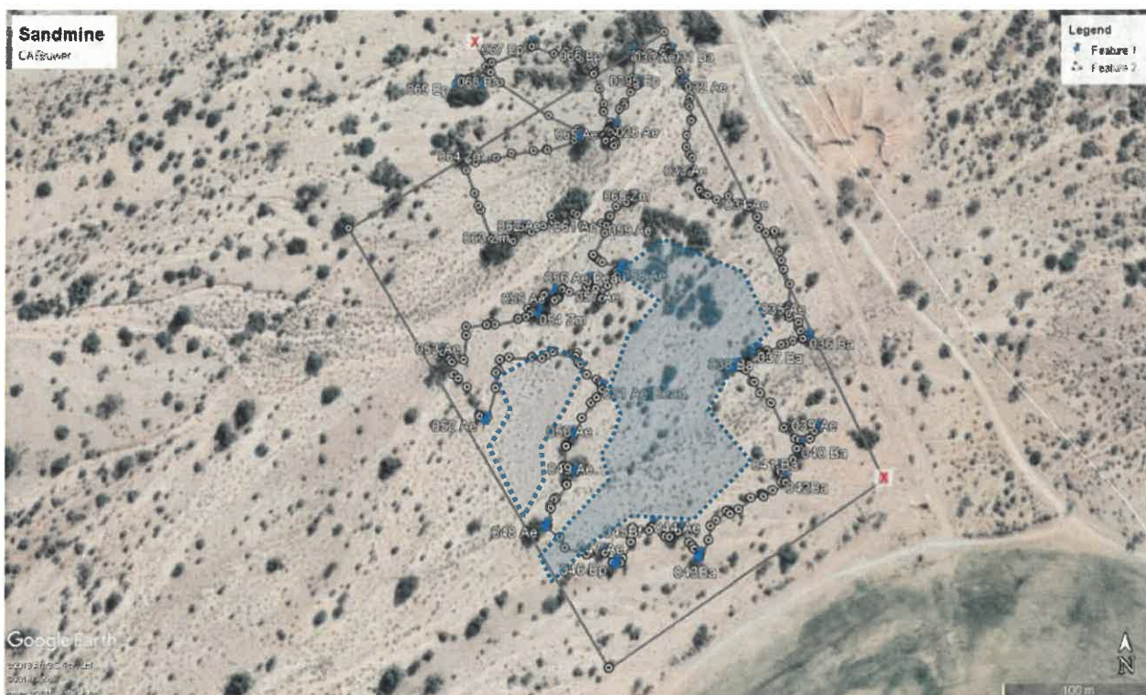
Figure 1: Potential areas for sand excavation as made by botanical/biodiversity specialist after initial botanical assessment. Grey outline indicates area investigated by specialists for potential borrow pit suitability.
