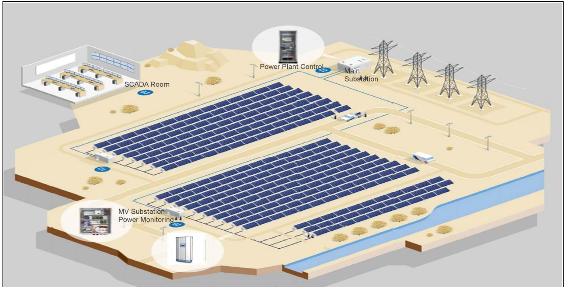
Figure 25: Representative typical arrangement of components in a conceptual PV development (as received from Cabanga Environmental, 2021).
