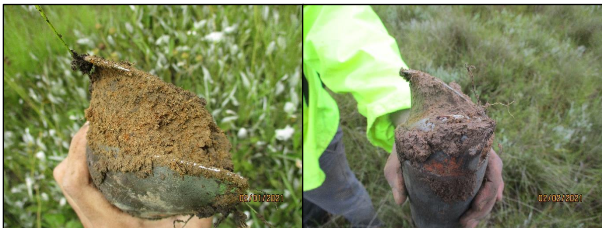
Figure 9: (Left) representative soil auger samples taken within UCVB wetland 1 indicating soil saturation, gleyed soil and mottling which serve as key indicators of a fluctuating water table.
