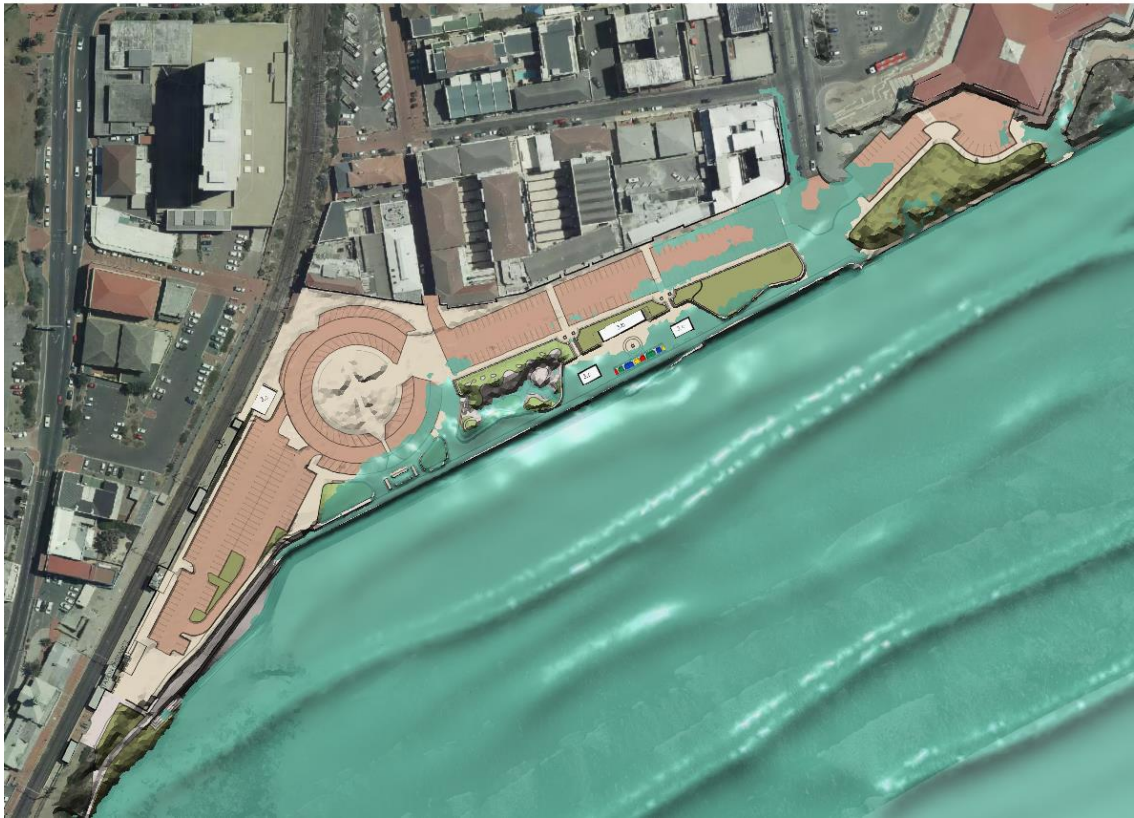
Figure 3-10: Instantaneous plot of surface elevation for the 100-year return period (100-year wave with a 1-year water level) and a 2076 climate change scenario.
