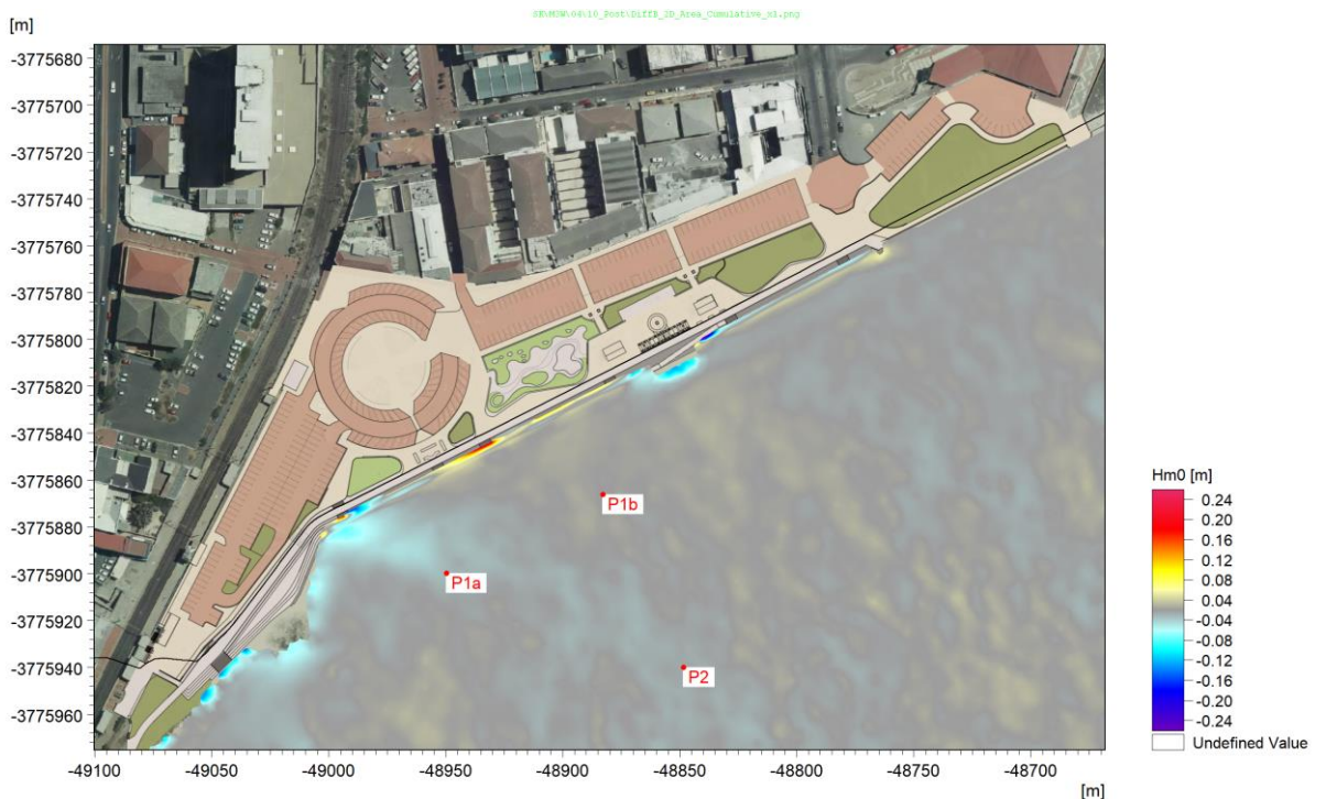
Figure 4-11: H_{m0} difference plot showing the difference between the proposed and existing seawall for wave Case B. A positive change indicates an increase in wave height for the proposed revetment.
