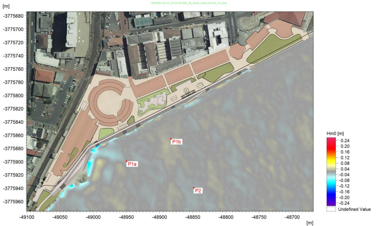
Figure 4-10: H_{m0} difference plot showing the difference between the proposed and existing seawall for wave Case A. A positive change indicates an increase in wave height for the proposed revetment.
