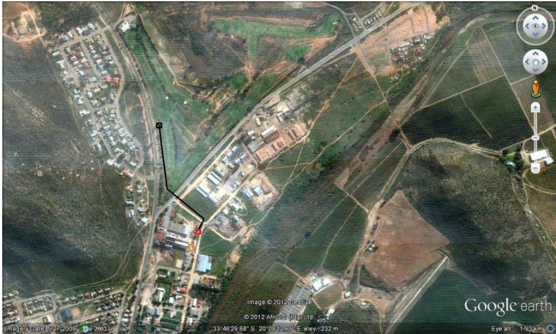
— Proposed pipeline from Montagu Cellar WWTW to Golf Course (to connect to current water supply system from Cogmanskloof Irrigation Board).
