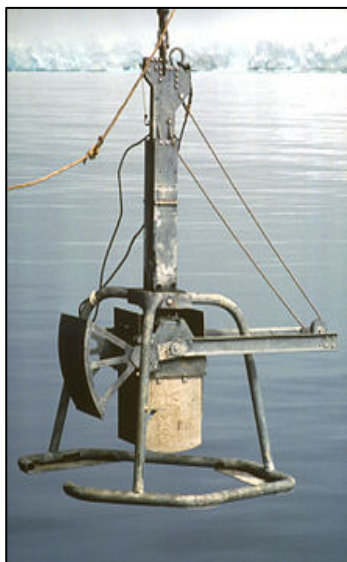
Figure 1.5: Box corer ( http://en.wikipedia.org/wiki/Box_corer ).
