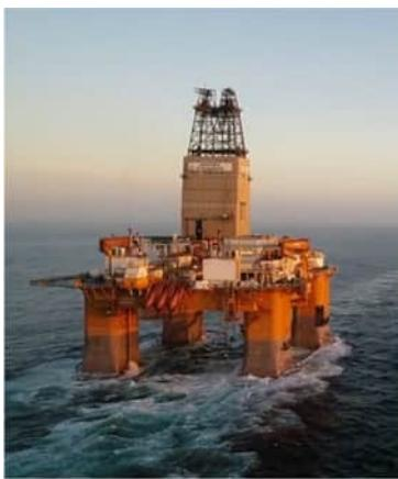
Figure 2: Semi-submersible drilling unit
