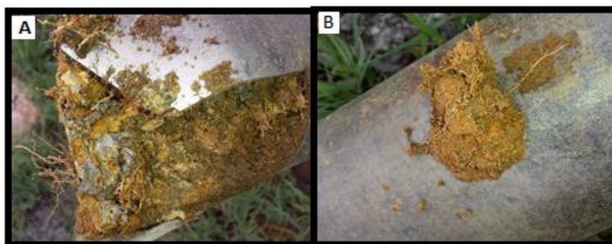
Figure 4-6: Soil form indicator (a) The quartzite layer at 30 cm (b) mottles in the soil
