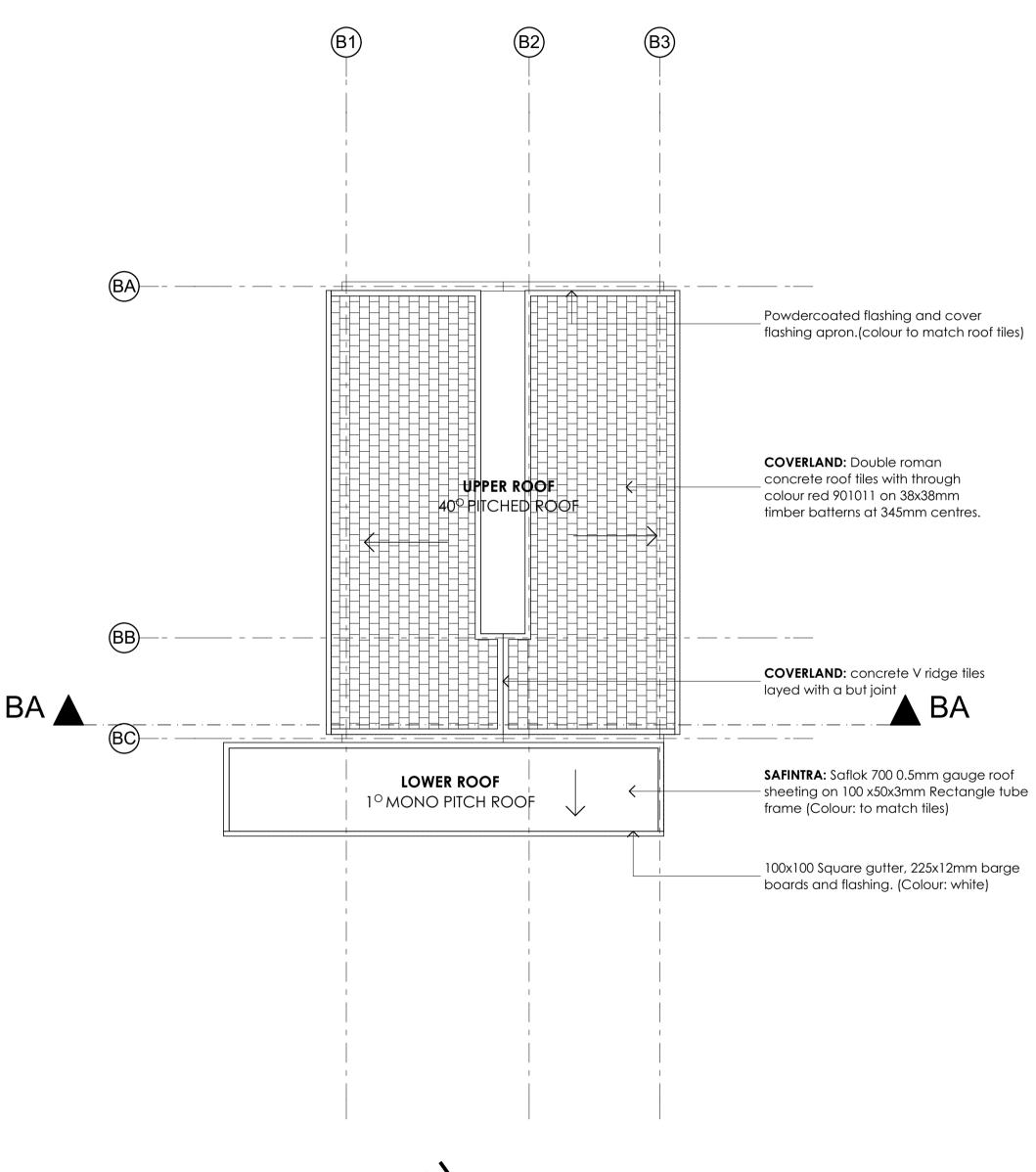
2. BLOCK B: ROOF PLAN Scale 1:100
