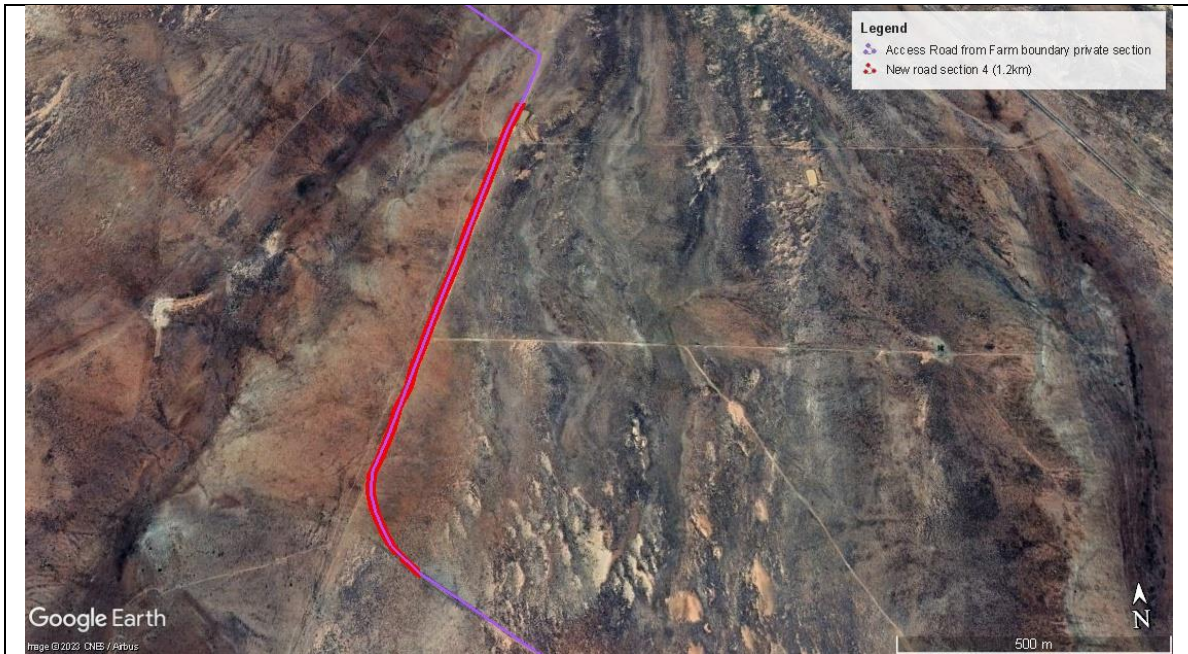
Figure 11. Road section 4 where the centre line of the proposed alignment is further than 5,5 m from existing farm tracks.
