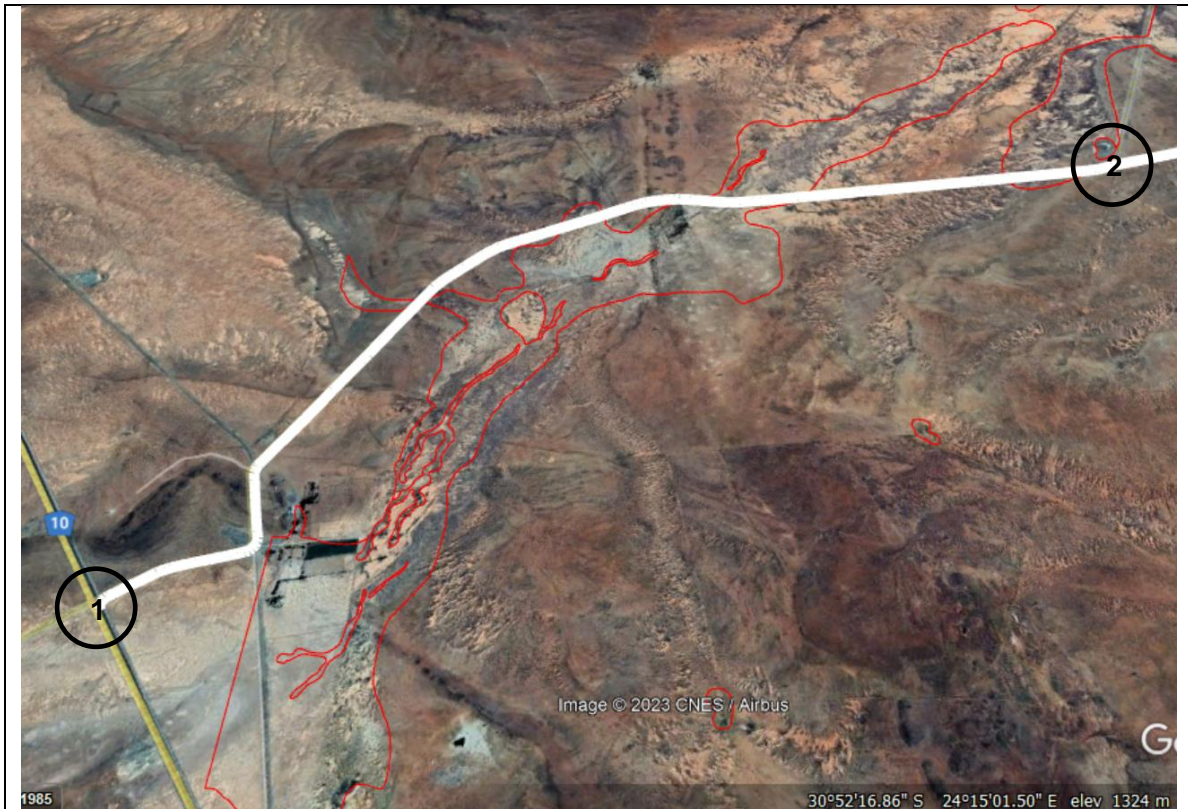
Figure 2. Section of existing public 'Burgerville' District Road (2448) from its intersection with the N10 (1) to its intersection with the existing private road (farm track) at the boundary of Farm Riet Fountain 39C (2). Red lines indicate flood plain soils (possible watercourses).
