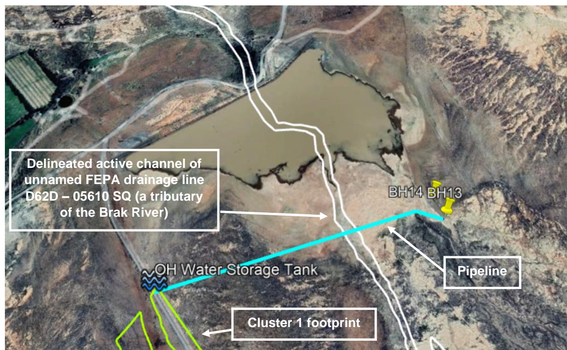
Figure 17. Route alignment of the underground 110 mm uPVC pressure pipe (blue line) from Boreholes No. 13 and/or 14 (BH13 & BH14) to the Overhead (OH) water storage tank inside the Cluster 1 footprint (delineated by the green lines).
