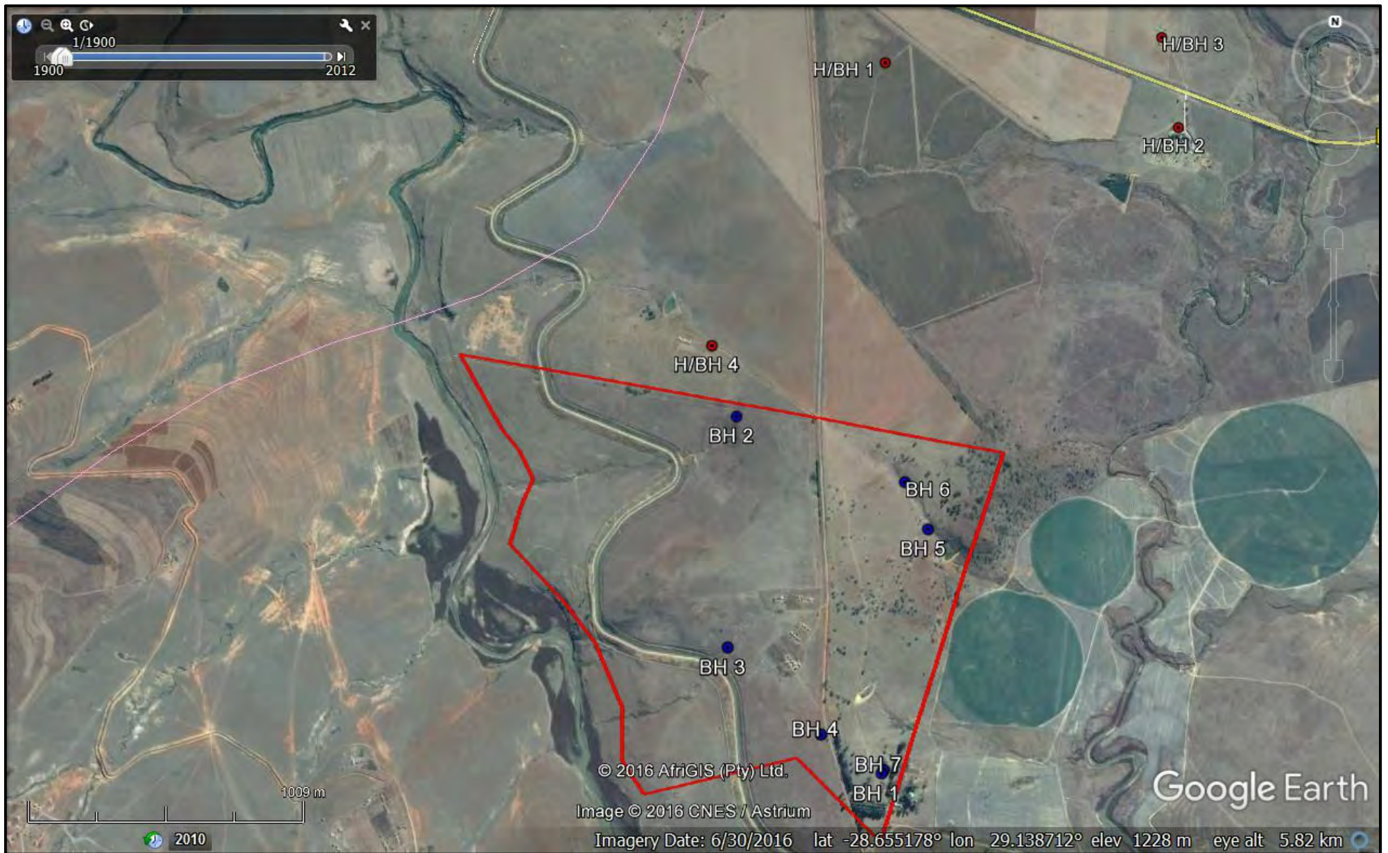
Figure 3: Hydro-census map. BH 1 is the existing borehole. Borehole BH 2 to BH 7 is newly drilled boreholes
