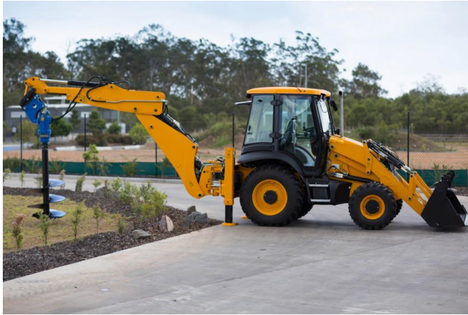
Figure 5: Example of a TLB mounted auger drill (Source: http://augertorqueusa.com )
