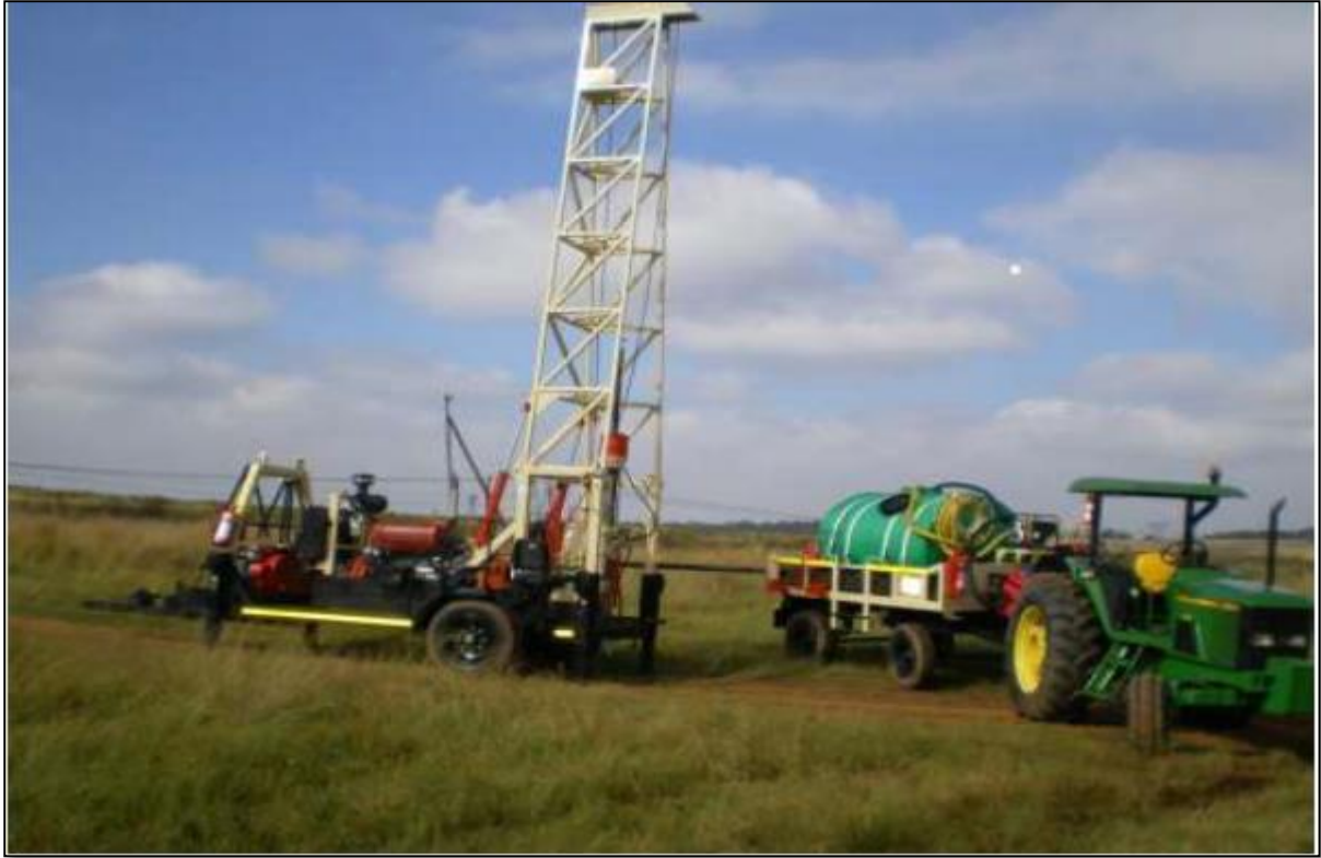
Figure 3-2: Typical LY44 Geological core drill unit
