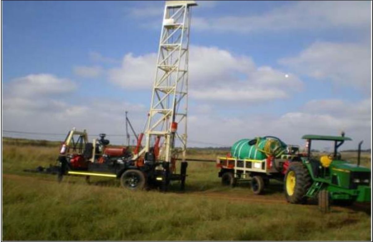
Figure 3-2: Typical LY44 Geological core drill unit
