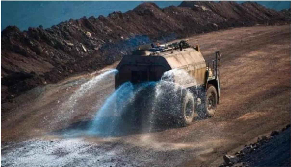
**Figure 46: Typical example of dust suppression using water truck.**
