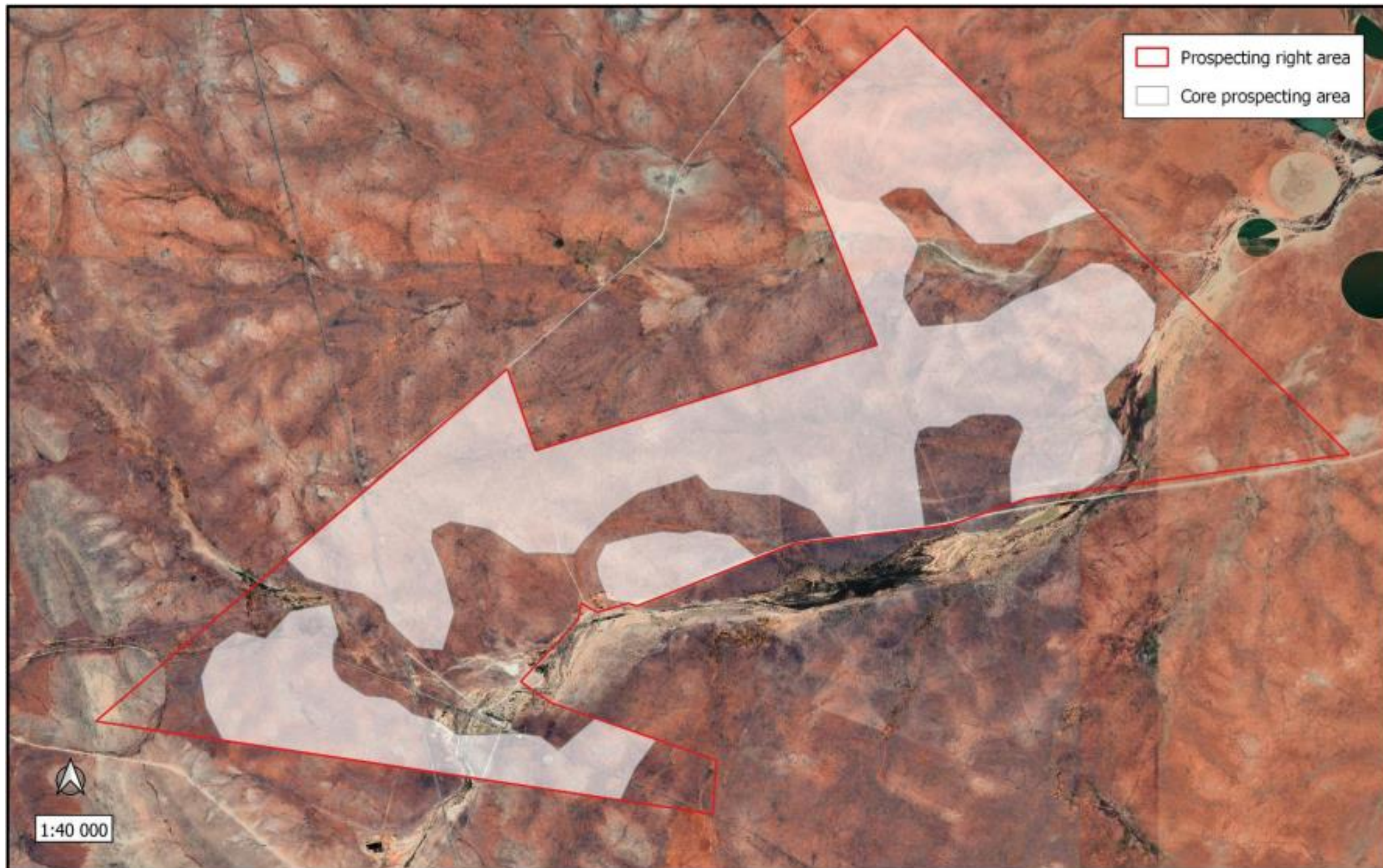
Figure 2. The prospecting area is indicated in red, with the proposed core footprint of prospecting activities indicated in white. The drill grid must still be established after mapping was completed (first non-invasive phase of prospecting planning).
