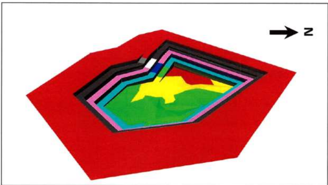
Figure 4. Schematic illustration of the pit design for the final push-back.
