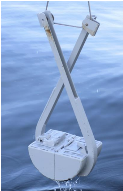
Figure 5. A Van Veen grab works like a claw to grab sediment containing macrofauna from the seafloor.
