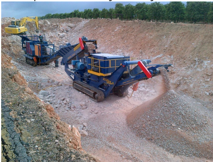
Photo 1: In-pit mobile tracked crushing and screening unit
