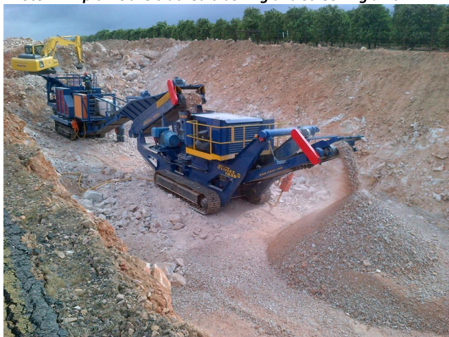
Photo 1: In-pit mobile tracked crushing and screening unit
