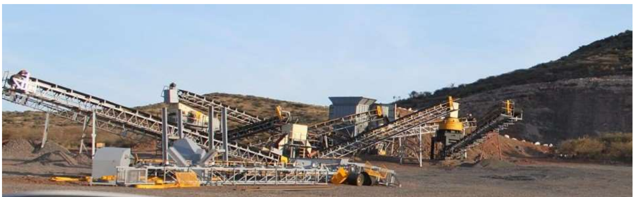
Photo 6: Crushing and screening Plant at the Gamohaan site during previous quarrying activities to be re-instated with upgrade.
