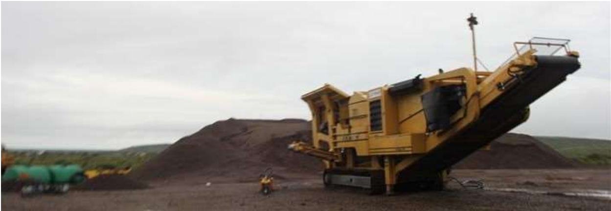
Photo 7: Typical in-pit tracked mobile primary crushing plant
