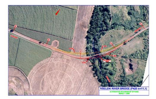
The preferred position is upstream from the current bridge as this provides for a future upgrade of the P425 with a Road Class 3 compliance of 100 km/h design speed and a smaller environmental footprint.
