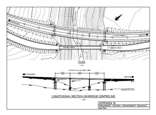
The bridge was designed so as to avoid placement of piers within the regular flow of the Nseleni River. Some temporary re-direction of the river and or construction of a temporary platform or a causeway may be required for the construction of the pier adjacent to the river.
