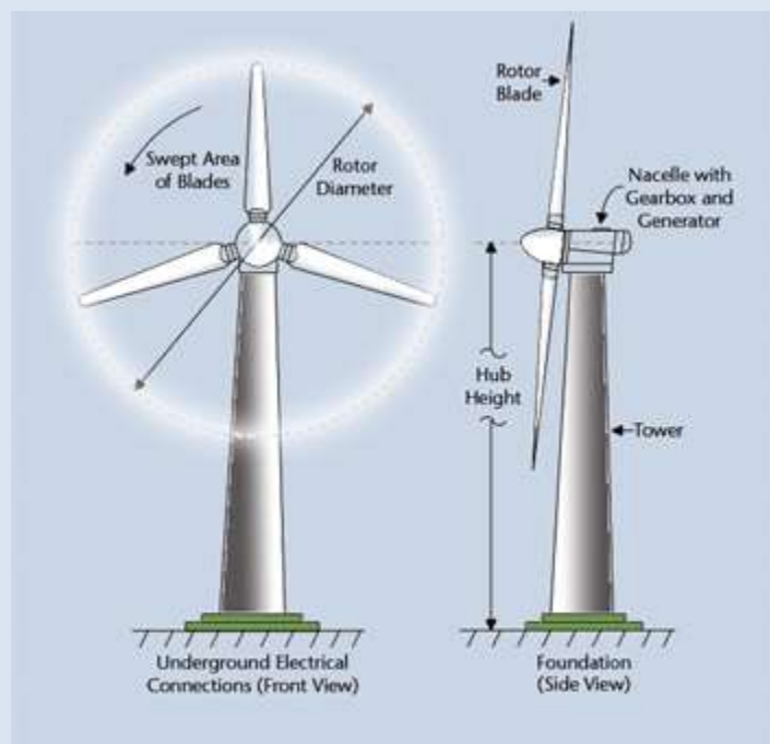
Drawing of the rotor and blades of a wind turbine, courtesy of ESN
