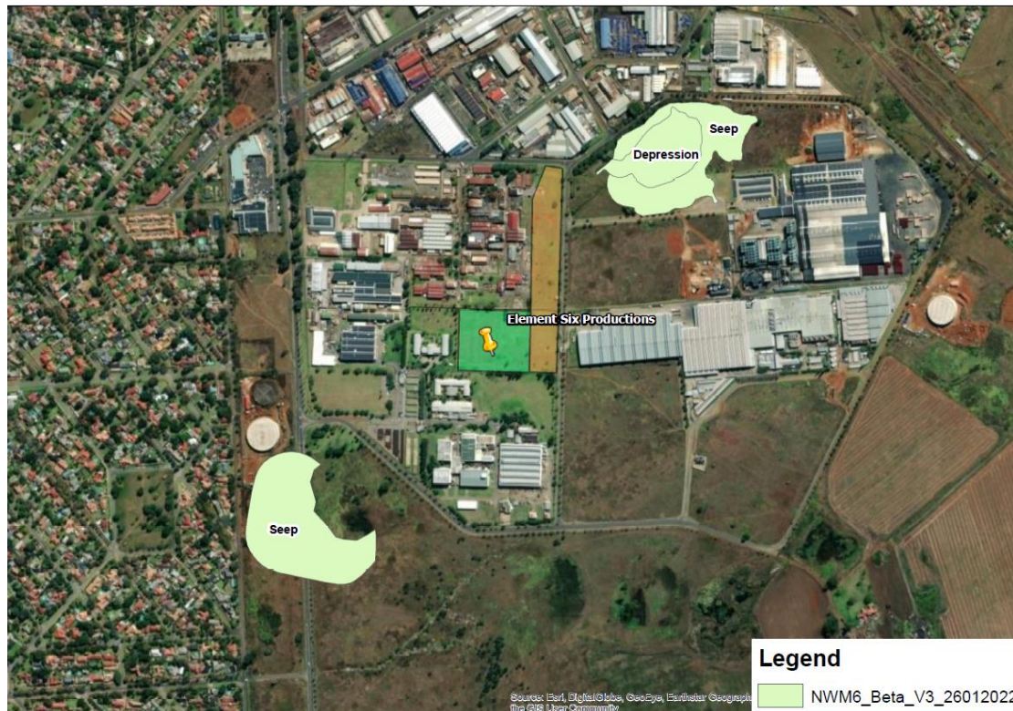
Figure 1. The proposed 2.2ha site (green polygon) for a 1.8MW Solar PV plant at the Element Six facility, Gauteng Province. Bioregional plan wetlands (light green polygons) occur to the south-west and north-east of the site. The orange polygon indicates a purported NFEPA wetland which has since been confirmed to be erroneous.
