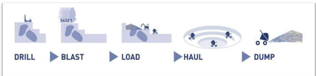
Figure 1: Process for open cast mining
