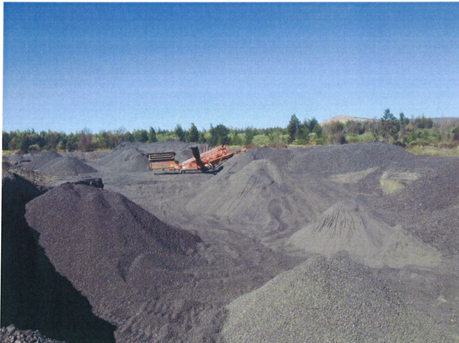
Photo 4: Bulk sampling trials producing screened “products” for testing
