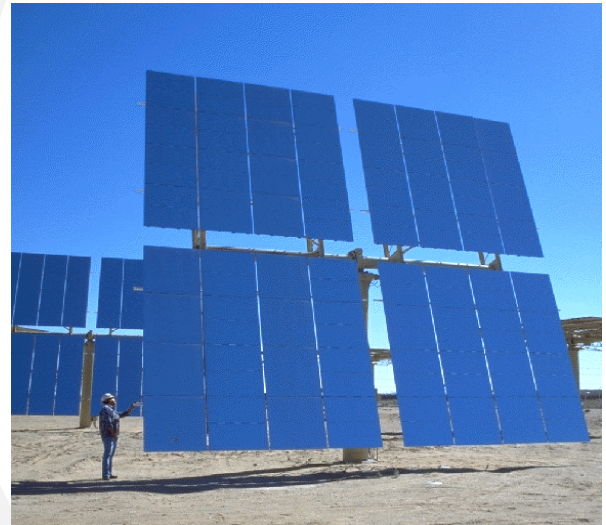
Figure 3: Single heliostat – image courtesy NREL
