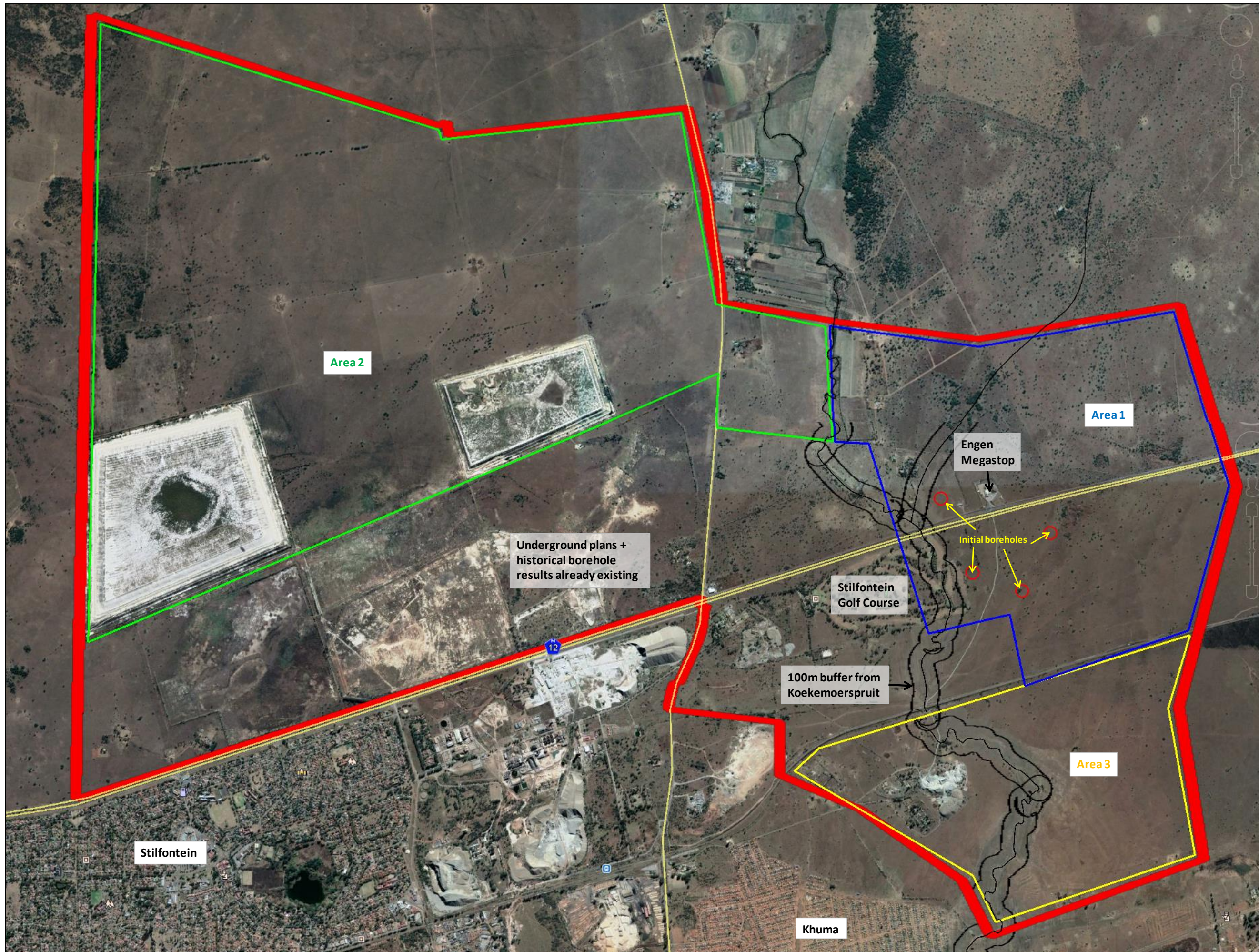
Figure 2: Indication of the preliminary positions of the initial 4 drill sites and the proposed further areas 1 - 3 for possible further drilling.
