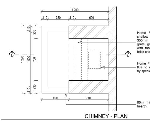
Home Fires model 700S single sided shallow built-in unit size 740 x 605 x 355mm deep made from mild steel, with grate, grid and ashpan, with coal scuttle, with toolset, with bolt-on fixed cowl for brick chimneymild steel.
