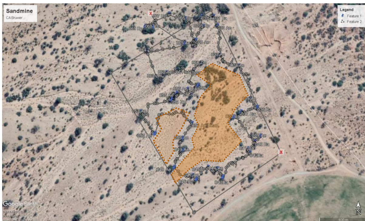
Figure 8: Proposed potential areas for sand mining, which will avoid the stream and protected tree species
