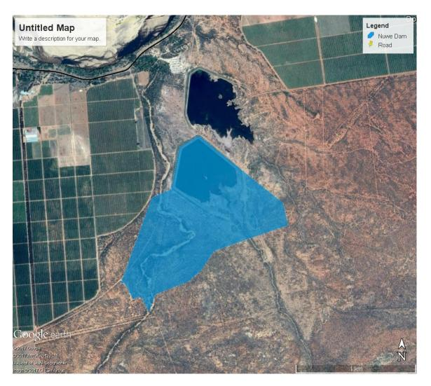
The proposed dam wall will be directly adjoining to the southern embankment wall of the existing dam and will extend to the south.
