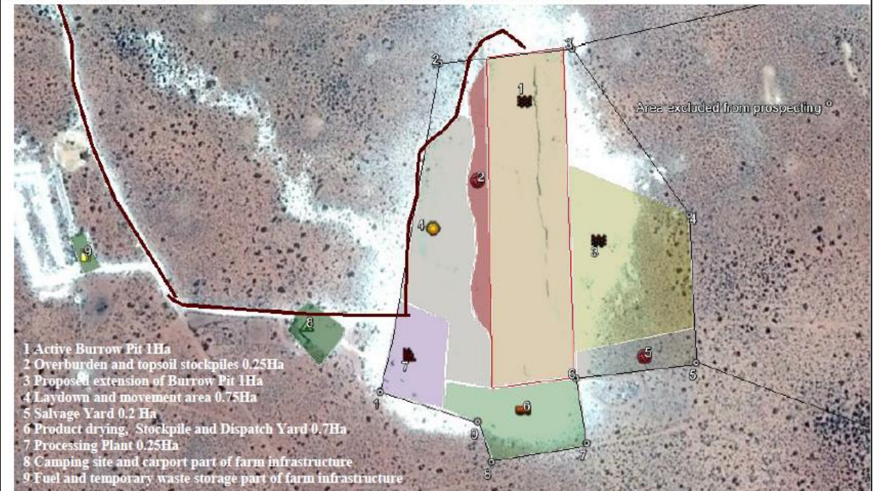
Diagram 3: Mine layout according to new footprint indicating logistical area and active mining area
