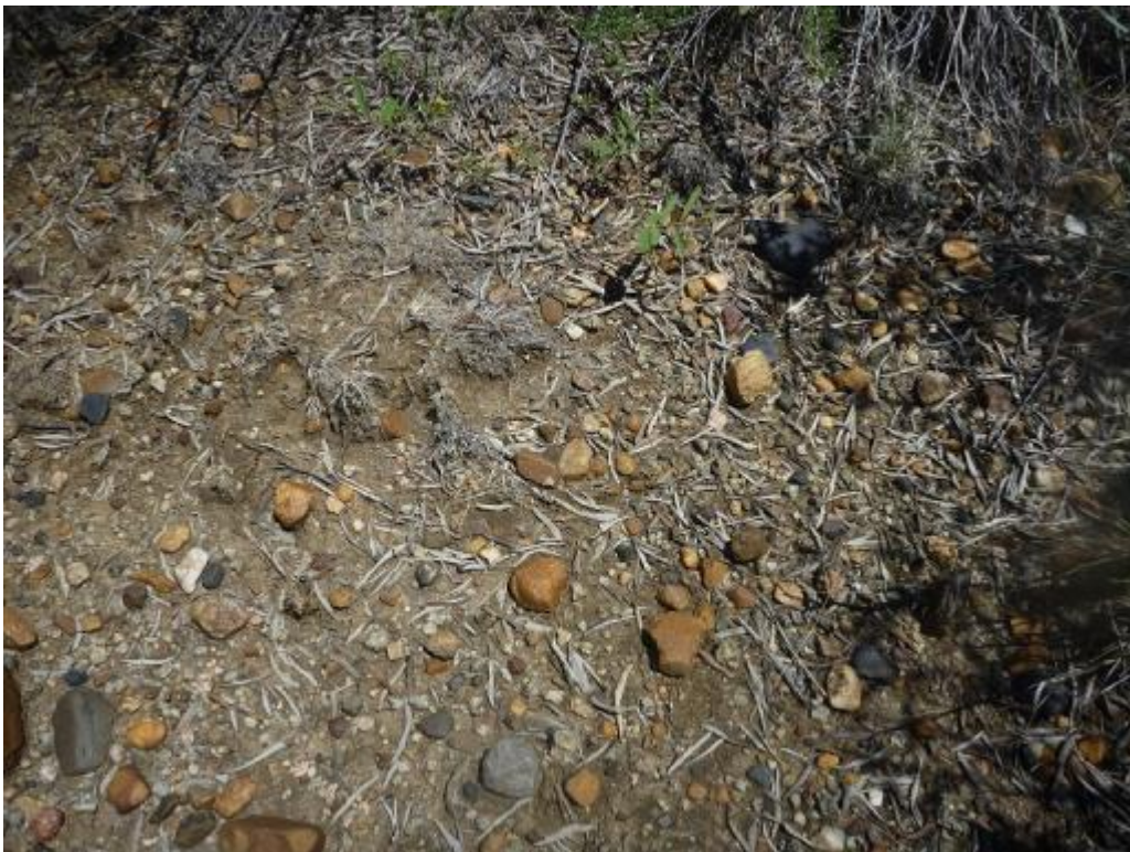
Figure 8 Rockiness on the soil surface of the soils of the Valsrivier soil form which are encountered towards the eastern section of the pipeline
