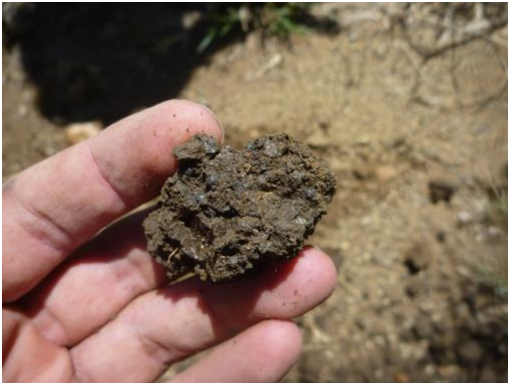
Figure 6 Blocky structure and clay illuviation in the pedocutanic B-horizon of the Valsrivier soil form
