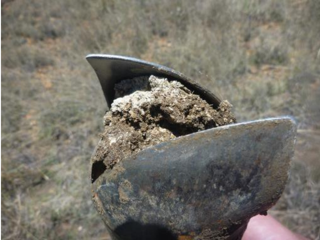
Figure 12 Calcification and weathering of rock in the non-diagnostic lithocutanic B-horizon that underlies the Arcadia soil form
