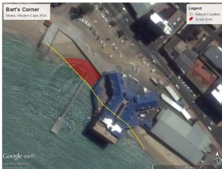
Figure 6: Aerial view of Bart's Corner. Yellow line – assumed natural coastline, red area – scour zone (Google Earth, 2017).
